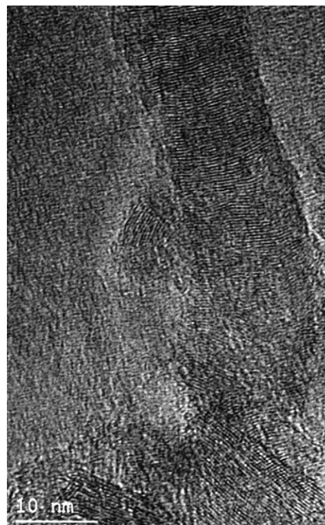
Fig. 8. TEM micrograph of carbon nanofibers obtained at 655 °C in C 2 H 6 :H 2 = 18:85 (120 ml (STP)/min) and detached from SMF Ni .
